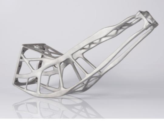
Lightweight and highly stable: The topologically optimized antenna bracket for Sentinel satellites with EOS Aluminium AlSi10Mg using additive manufacturing. (Source: EOS GmbH)
