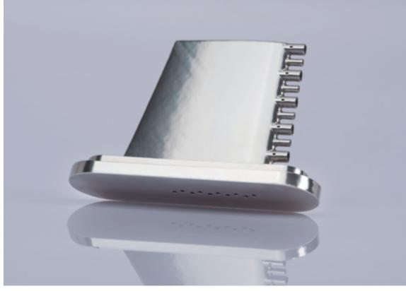
Extremely rigid and durable: this compact flow measurement probe was made in one piece using industrial 3D printing (source: EOS GmbH, Vectoflow).
