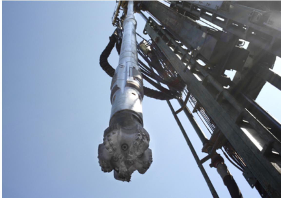
Drill bit and rotary steerable system (RSS): Complex parts for rotary steerable systems, which actively steer oil and gas wells, are now being produced by APS Technology, Inc. using industrial 3D printing technology from EOS. (image courtesy APS)
