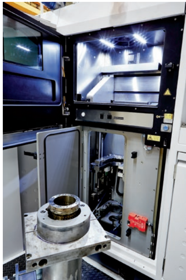
EOSINT M 280 Custom: The system was individually adapted to Siemens requirements and helps simplify and speed up the repair procedure of burners for industrial gas turbines (Source: Siemens).
