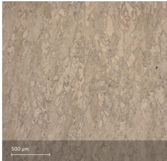
Microstructure solution annealed Etched with etchant Kallings 2
