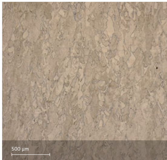
Microstructure solution annealed Etched with etchant Kallings 2
