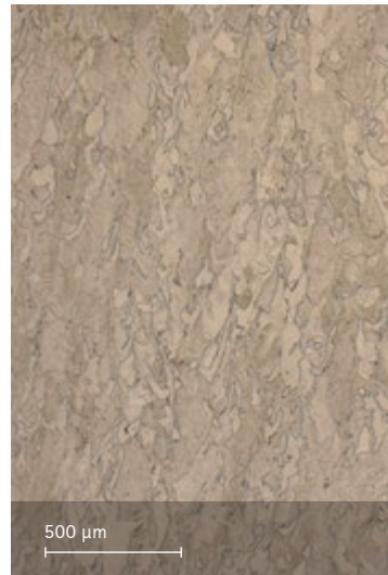
Microstructure solution annealed Etched with etchant Kallings 2
